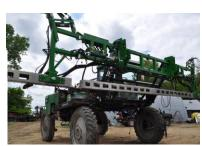
**Durability:** Sprayflex Aluminum Box Boom design allows the booms to "flex" without fatigue unlike competitors welded aluminum and steel booms.
